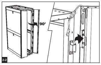
Loosen the screws Lattaching the hinge swivels L to the vertical sections in the four locations indicated. You will retighten the screws in the next step, after attaching the frame to the rack enclosure.
